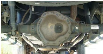
**Axle Ratio:** The rear axle is also referred to as the differential or final drive. The axle is what actually makes the vehicle move. The vehicle's engine creates power and torque but you need to get that power to the wheels. To do that the power from the engine goes to the transmission and from there back to the differential or axle. Inside the axle gears multiply the power and send it to the drive wheels, making the vehicle move. When a manufacturer
